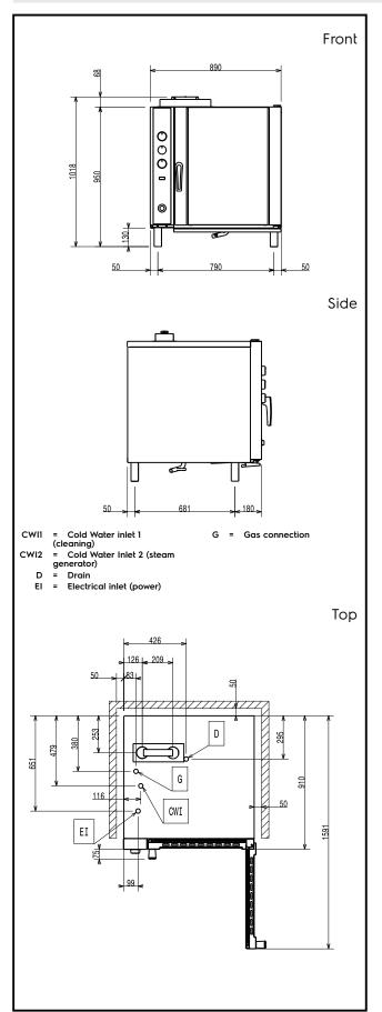
Electric Supply voltage: 220-230 V/1 ph/50 Hz 0.35 kW Auxiliary: Electrical power, max: 0.35 kW Gas Gas Power: 18.5 kW Capacity: Trays type: 10 (GN 1/1) **Key Information:** External dimensions, Width: 890 mm External dimensions, Depth: 900 mm 970 mm External dimensions, Height: Net weight: 136 kg Functional level: Basic Cooking cycles - air-convection: 300 °C Internal dimensions, Width: 590 mm Internal dimensions, Depth: 479 mm Internal dimensions, Height: 680 mm **ISO Certificates**
